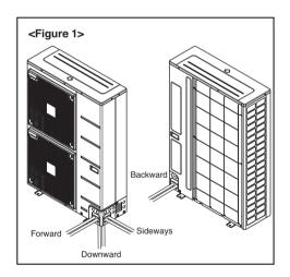
When connecting in a downward direction, knock out the knock-out hole of the base pan. (refer to figure 2)
